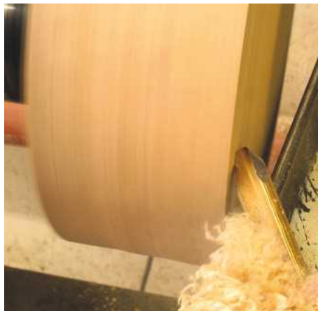
▲ Pic.5 Use the 13mm bowl gouge in a pull cut to remove the bulk of the unwanted wood from the area around the foot. Keeping the tool handle low will help the tool to cut rather than scrape
